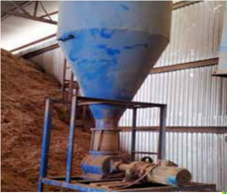
Hammer Mill - Ensures uniform particle size for making the briquettes.
