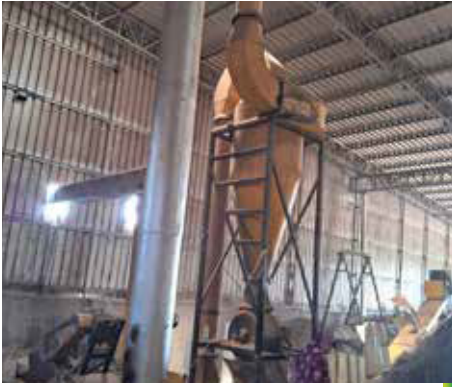
Dust Remover - Reduces ash content in raw materials.
